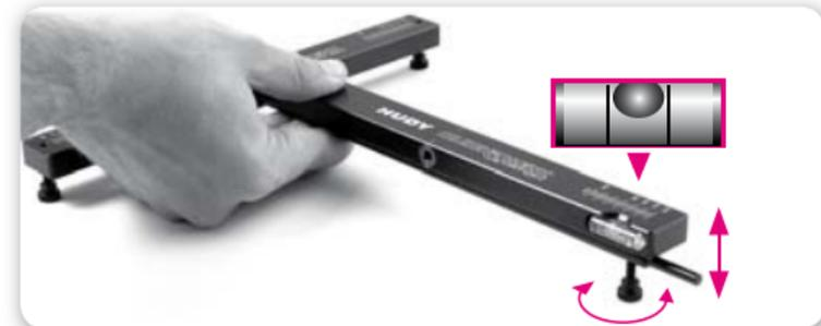
**Center Axle:** Lay the pivoting base plate along the top of the center axle so you can observe the spirit level. Adjust the threaded foot in the center axle until the bubble in the spirit level is between the middle lines.
