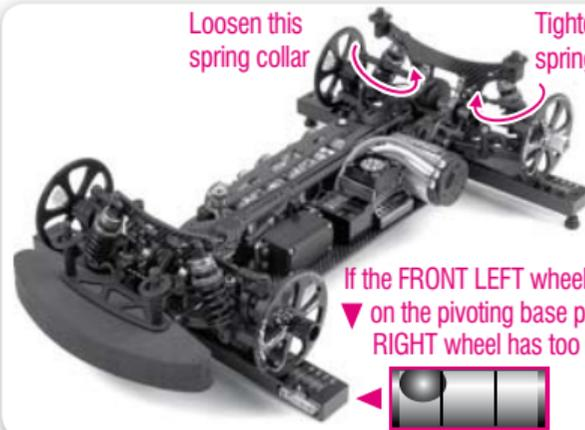
If the FRONT LEFT wheel pushes down on the pivoting base plate, the REAR RIGHT wheel has too much tension.
